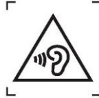
Figure 1 – Warning label (IEC 60417-6044)
